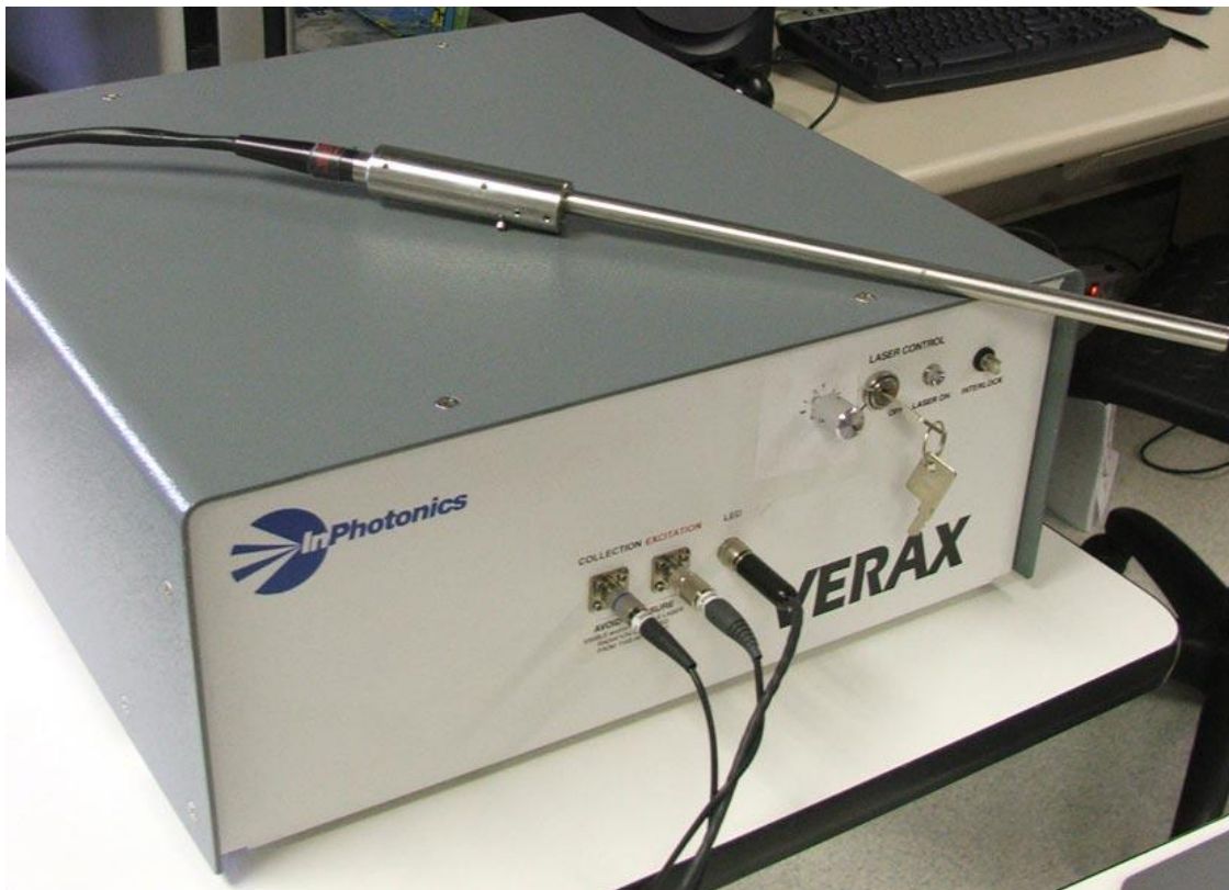
Figure 2-2: A Raman probe attached to an InPhotonics portable Raman spectrometer
