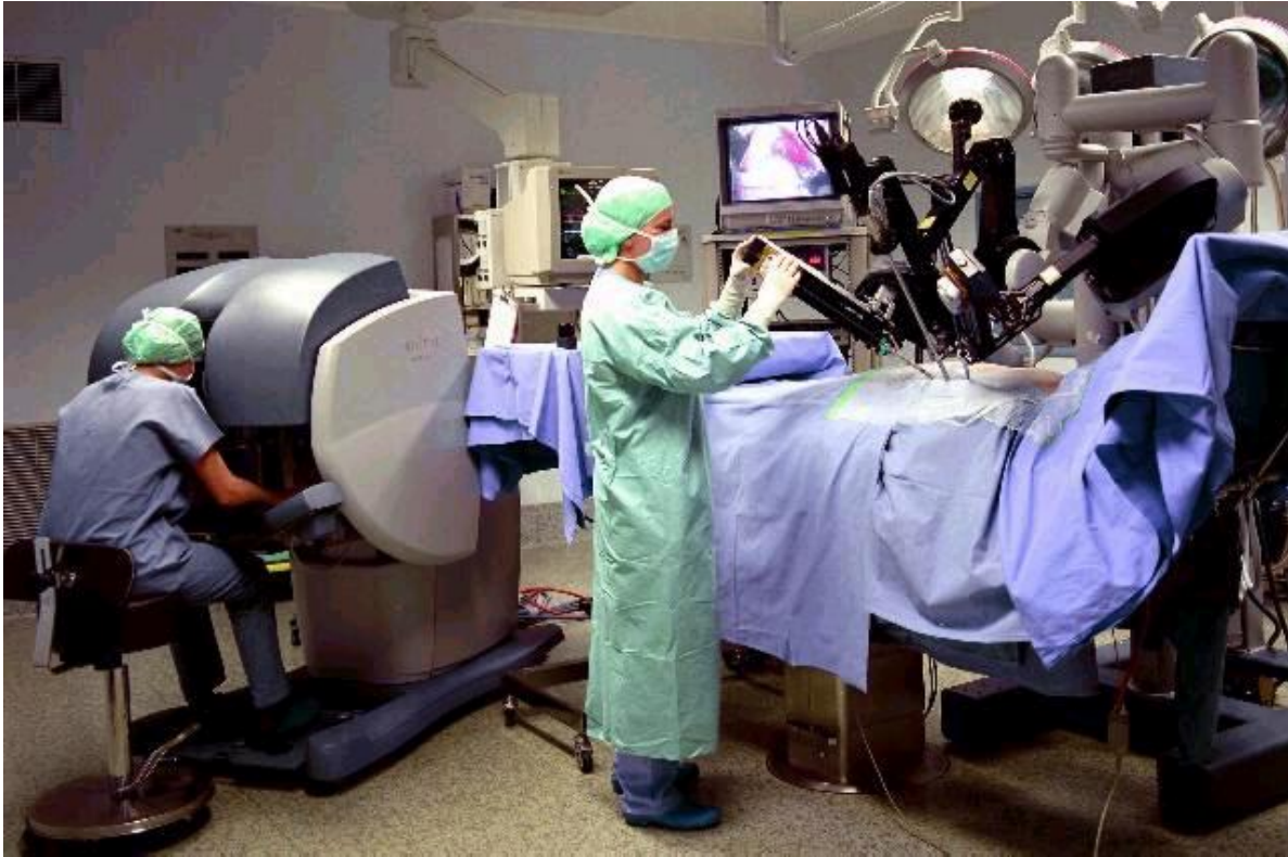
Figure 2-4: The da Vinci surgical system. The surgeon sits at the control station on the left, while the tools are inserted into the patient on the right. Image © 2011 Intuitive Surgical, Inc.
