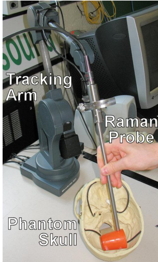
Figure 6-1: The Raman probe, attached to the end of the MicroScribe G2X, is used to scan a plastic cup and other objects with the phantom skull
